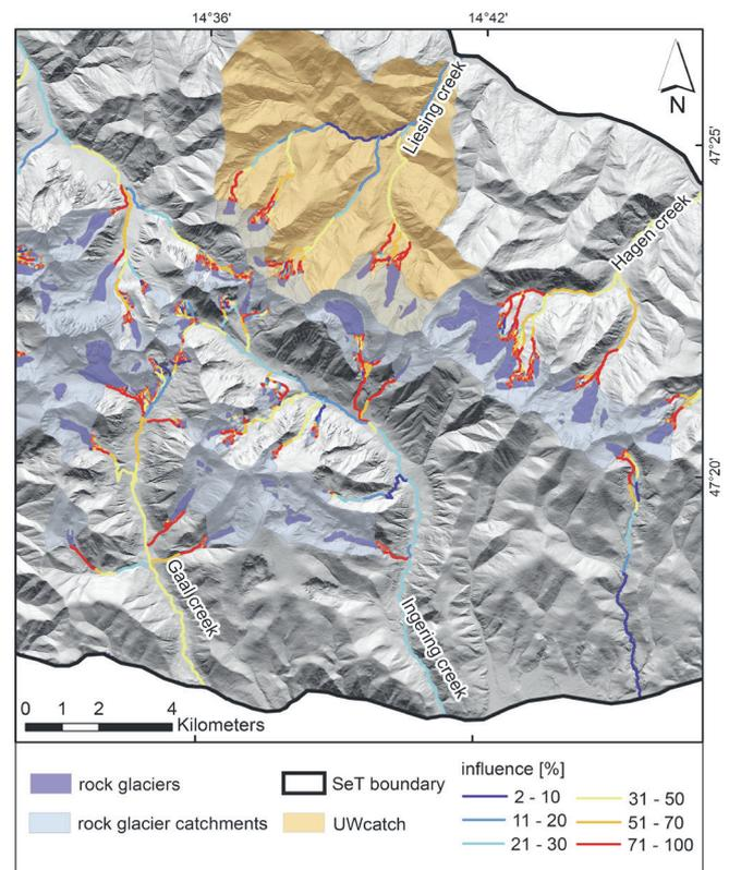
**Figure 3:** Runoff contribution map of the area: considering long-term runoff estimates based on a simple water balance ( $Q = \text{precipitation (P)} - \text{evapotranspiration (ETa)}$ ); the proportion (in %) of water draining relict rock glacier bodies are displayed along the downstream stream network approaching the main valleys. The Unterwald catchment (UWcatch) is highlighted in orange.
