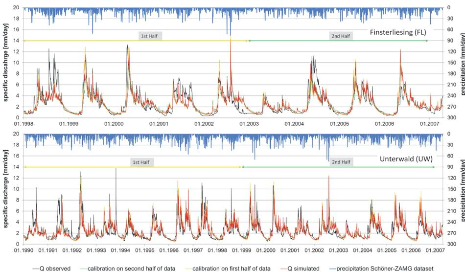
**Figure 7:** Observed and simulated runoffs of FL and UW using GR4J+. Observed discharge is compared to simulated discharge based on calibration on different parts of the data and the related validation is shown.
