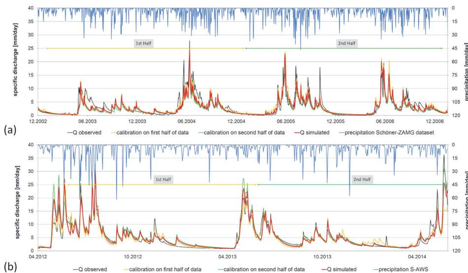
**Figure 5:** Comparison of observed and simulated runoff of SEQ using the GR4J+. Observed discharge is compared to simulated discharge based on calibration of different parts of the data (complete data set, first and second half) and the related validation is shown. For the time period 2002-2007, the forcing input (precipitation and air temperature) is based on the Schöner-ZAMG dataset (a); for the time period 2012-2014, the data from the S-AWS weather station is used (b).
