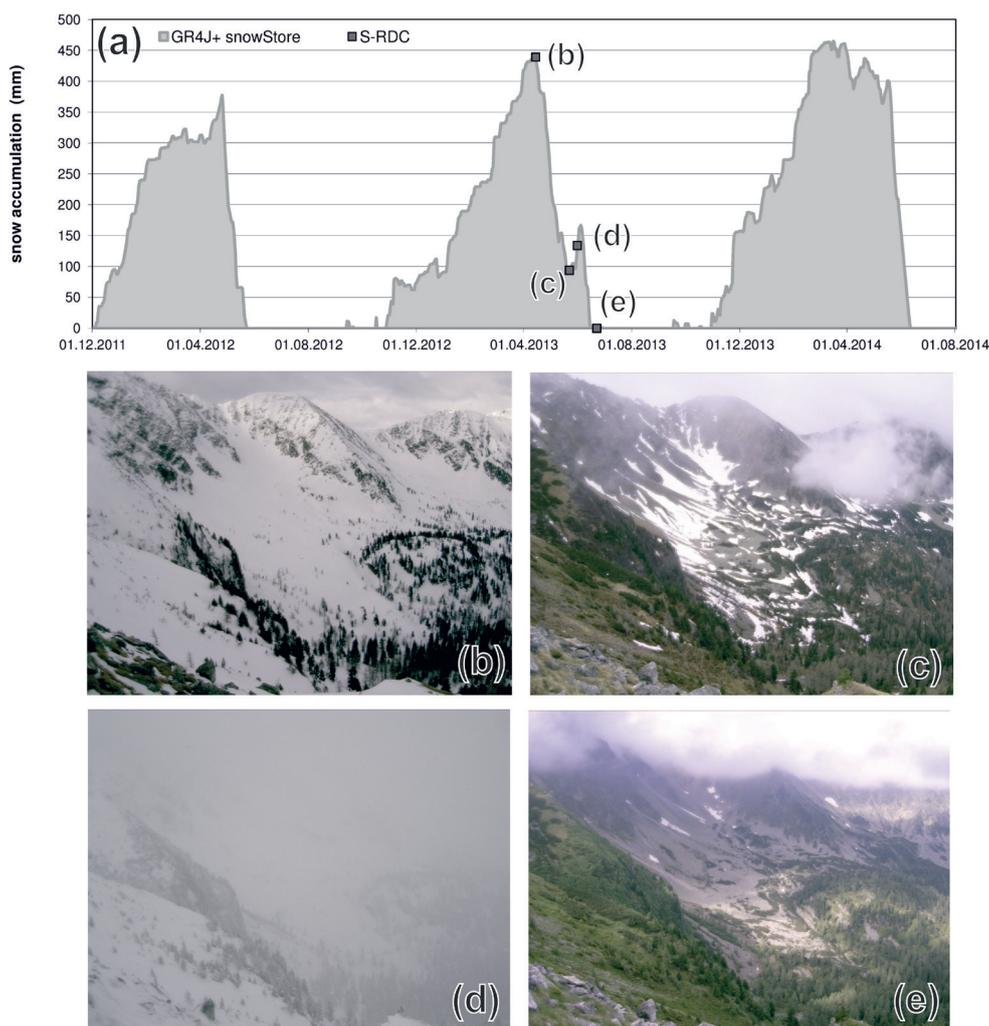
**Figure 6:** Comparison of snow model results and observed snow cover. (a) Modeled snow accumulation for the SRGcatch. Note the snow melt periods especially in May and June. (b-e) Extend of snow cover based on pictures of the S-RDC correlate well with the modelled snow accumulation and melt as indicated by exemplary photos related to certain time periods indicated in (a).
