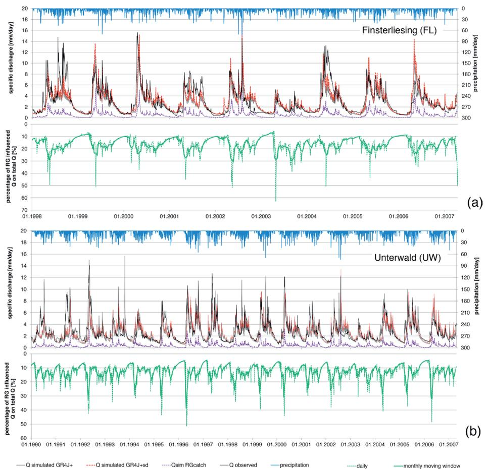
**Figure 9:** Observed and simulated runoff of Finsterliesing (FL) (a) and Unterwald (UW) (b) gauging stations. Simulated runoff based on the semi-distributed (GR4J+sd) and the fully lumped (GR4J+) approach and the simulated runoff from the respective rock glacier-influenced headwaters (Qsim RGcatch) is shown. In addition, the percentage of relict rock glacier (RG)-influenced headwater-runoff compared to the total runoff on a daily basis and using a one month moving window is displayed.
