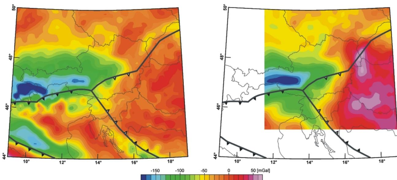
**FIGURE 4:** (a) Bouguer gravity (BA) compiled from Bielik et al. (2006) and from data supplied by the West\_East Europe gravity project (<http://www.getech.com>); (b) BAC, the gravity effect of density variations in the upper crust stripped (Simeoni and Brückl, 2009); the plate and country borders are superimposed on both maps for orientation.
