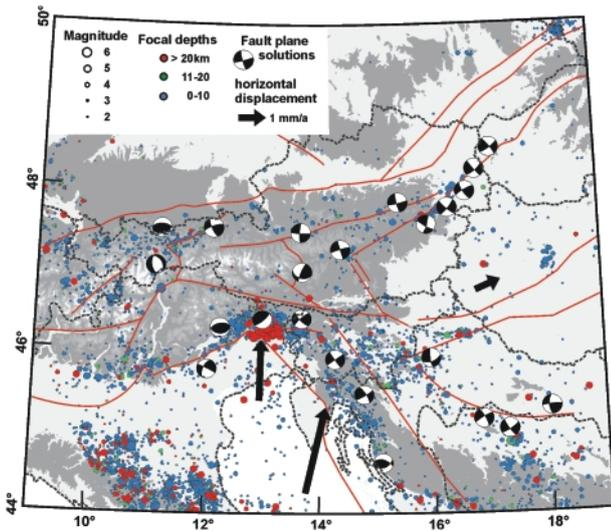
**FIGURE 6:** Active tectonics documented by seismicity and plate velocities. Major faults, seismicity (NEIC, 1973-2008), and representative focal plane solutions (see Brückl et al., 2010 for references) are superimposed on digital terrain model. Arrows show horizontal plate velocities derived from GPS-data (Grenerczy and Kenyeres, 2006; Weber et al., 2006) relative to Europe.
