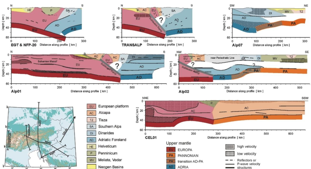
**FIGURE 2:** Modern seismic cross sections in the wider Eastern Alps area (modified after Brückl, 2010). The cross sections show the major seismic structures, the geological units of the upper crust, and a tentative attribution of the middle and lower crust to the major tectonic plates or blocks (Adria, Europe, Pannonian domain). For references and particulars please see chapter: Geophysical traverses across the Eastern Alps and the surrounding areas.
