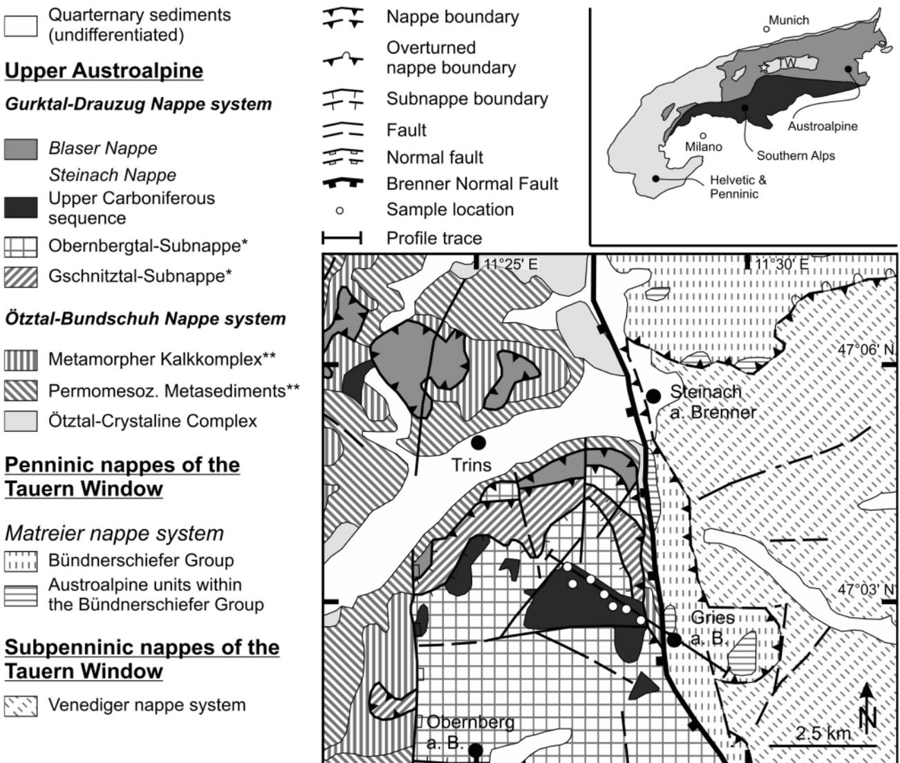
**FIGURE 1:** The inset shows the major structural units of the Alps. A star indicates the study area at the western termination of the Tauern Window (TW). The simplified geological map of the working area shows the major geological units, the sample localities and the profile trace. \*) These subnappes together form the Steinacher Quartzphyllite. \*\*) Together these units form the Brenner Mesozoic (BM). (after Rockenschaub & Nowotny, 2009)
