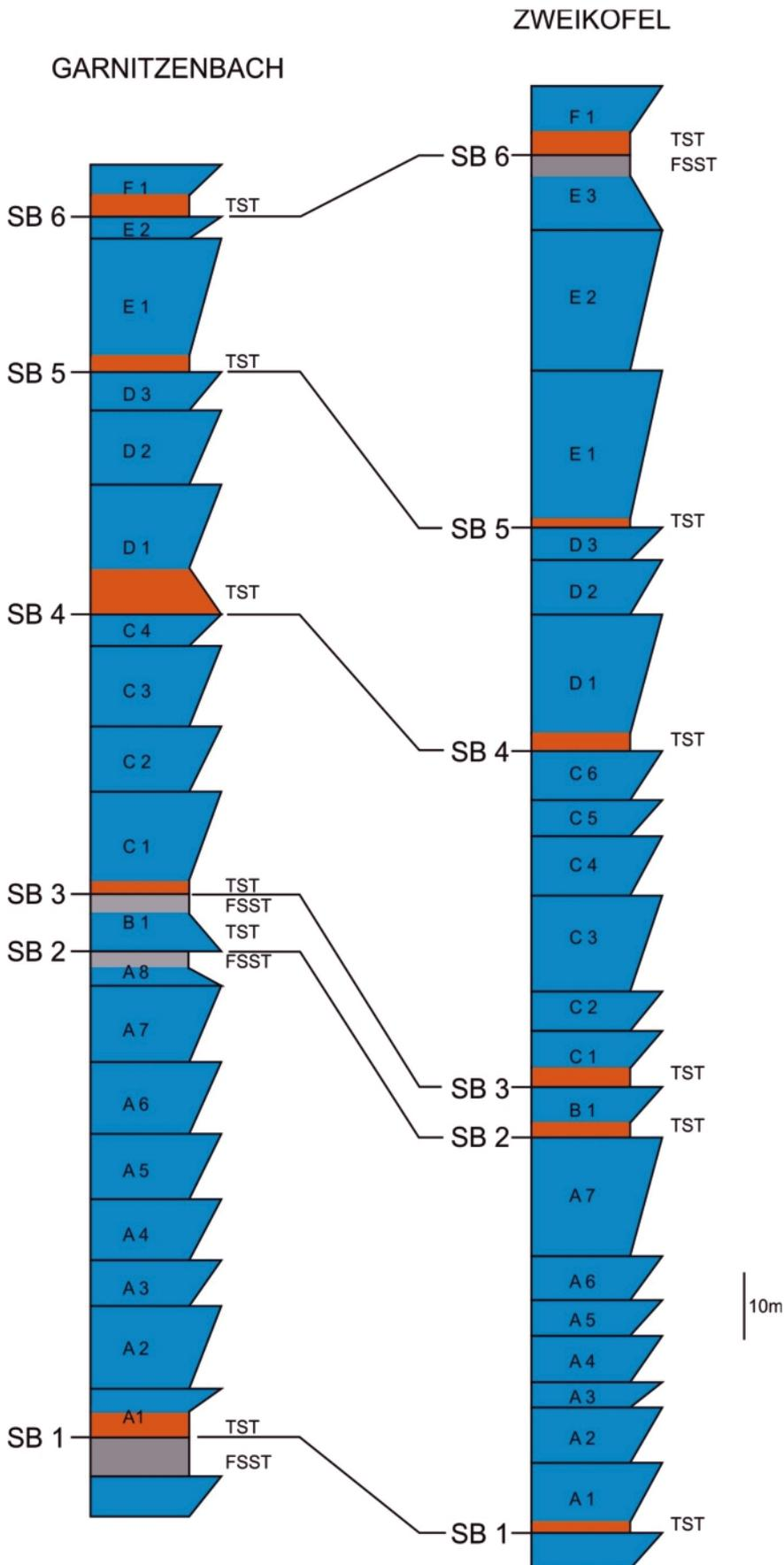
**FIGURE 12:** High-frequency cycles (parasequences) of the Zweikofel Formation at Garnitzenbach and Zweikofel. Blue: limestone parasequences, shallowing upward, grey: thin siliciclastic horizons interpreted as falling stage systems tracts (FSST), orange: siliciclastic horizons interpreted as transgressive systems tracts (TST). SB: sequence boundaries.
