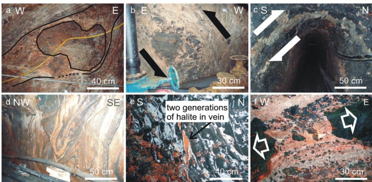
**FIGURE 18:** Altaussee, style of deformation and reverse faulting of foliation. (a) Stream line body around rigid object. (b) Circumfluent shale clast, folds in adjacent rocksalt. (c) View along gallery towards W. Layer of sandstone in mudrock matrix. (d) Isoclinal folds in rocksalt. (e) Veins in mudrock, filled with inner red and outer white halite. (f) Non-rotation deformation with strain shadows filled with white halite in red halite matrix.
