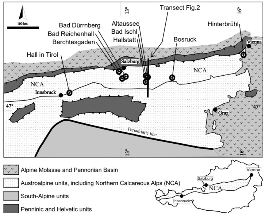
**FIGURE 1:** Overview sketch map of the Eastern Alps. Main tectonic units and location of salt mines in the central NCA. Insert at right bottom gives the position within Austria. Circles mark rocksalt deposits.
