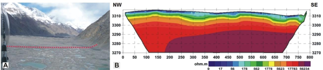
**FIGURE 6:** Oblique view of the Peremitschka to northeast (photo taken by Häusler from helicopter on 8 May, 2009). After the outburst of Lower Lake Merzbacher, glacier karst features and countless depressions filled up with water from melting icebergs are visible (A). The ERT profile crosses the Northern Inylchek Valley in a northwest-southeast direction at an altitude of 3320 m a.s.l., and shows resistivities of up to 100.000 ohm.m (B).
