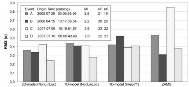
**FIGURE 8:** RMS error for travel-time residuals of the four selected events from the three locations methods. The best adaption of travel times is observed by the nonlinear algorithm in combination with the 3D-model (P- and S-waves).
