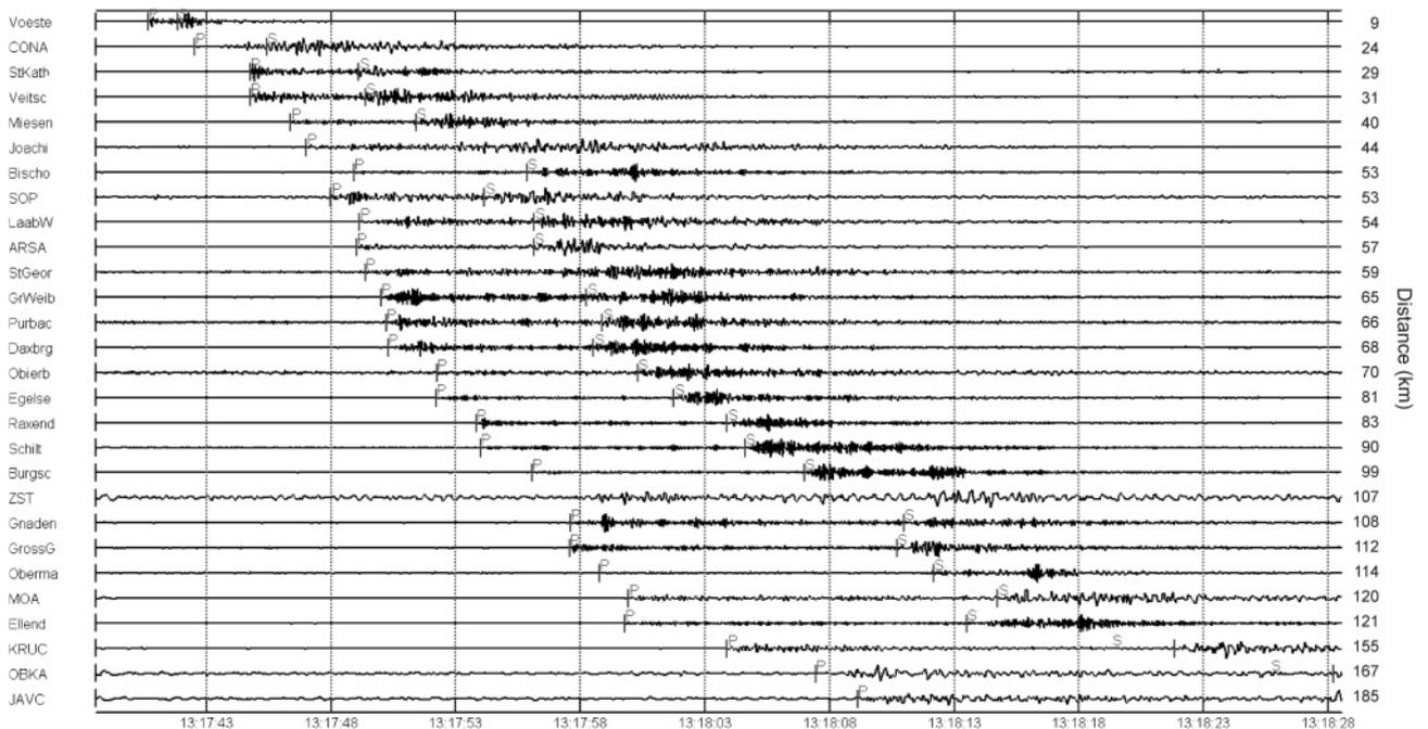
**FIGURE 7:** Example B of seismic data recorded at the Z-component and sorted by the epicentre distance from the bulletin. The magnitude MI = 2.2 event occurred on 2006 04 15 13:17:38 and was located from ZAMG to be in the west of Neunkirchen (Fig. 2). The data were processed with frequency band-pass filter (1 – 12 Hz) and span a period of 50 seconds.
