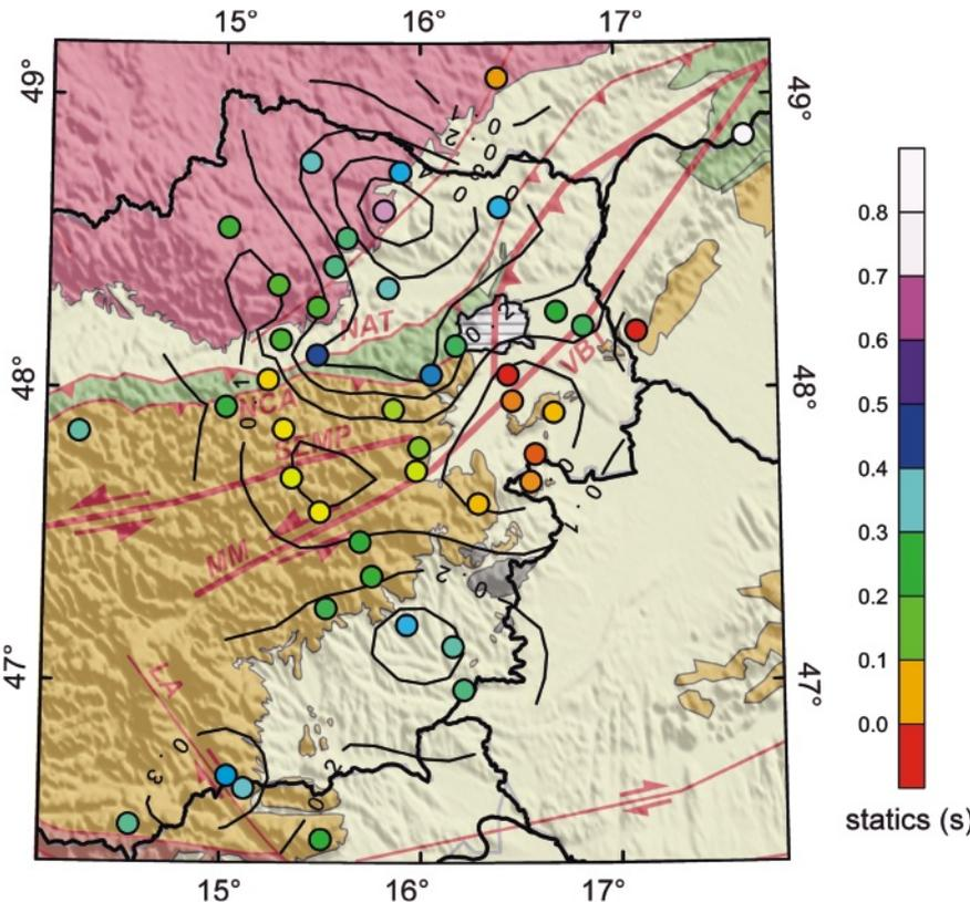
**FIGURE 6:** Preliminary station corrections for P-wave times for the 3D velocity model displayed as contour lines and symbols (coloured circles) over the major geological and tectonic structures of the Eastern Alps. LA (Lavantal fault), NAT (North Alpine Thrust), NCA (Northern Calcareous Alps Thrust), MM (Mur-Mürz fault), SEMP (Salzach-Ennstal-Mariazell-Puchberg fault).
