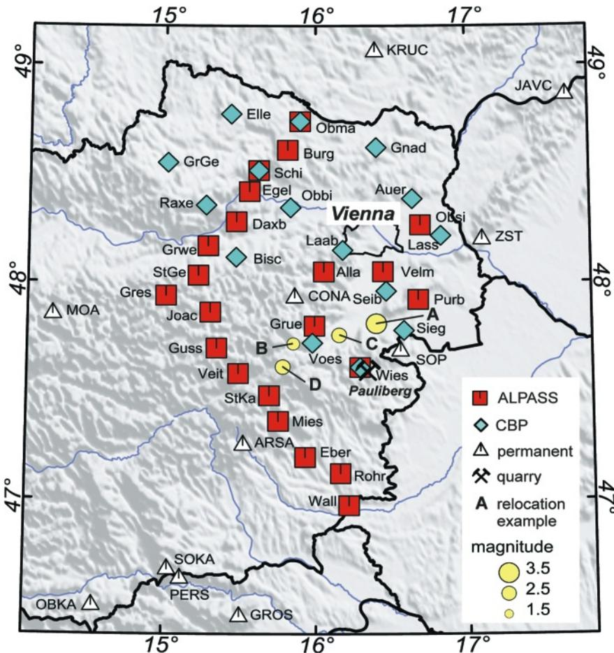
**FIGURE 2:** Location of temporal (ALPASS and CBP) and permanent seismic stations used for this study. Characters A, B, C, and D identify epicentres of earthquakes which were analyzed to find the best location method. The quarry Paulberg used for validation of the absolute location accuracy is also shown in this map.
