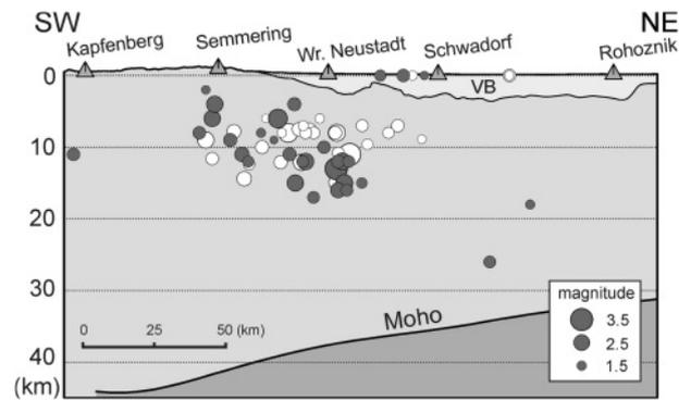
**FIGURE 11:** Crustal cross section of hypocentres along the MM fault and the VBT (for location, see Fig. 10) with the Vienna Basin (Miocene) (after Wessely, 1993) and the Moho (after Behm et al., 2007). In contrast to the routine locations (white) the new hypocentres (dark grey) display focal depths which get deeper towards NE.
